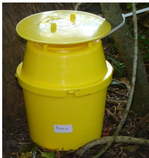
Figure 4.3: Trap made of one colour (yellow bucket, dome lid and funnel) for field bioassay.
