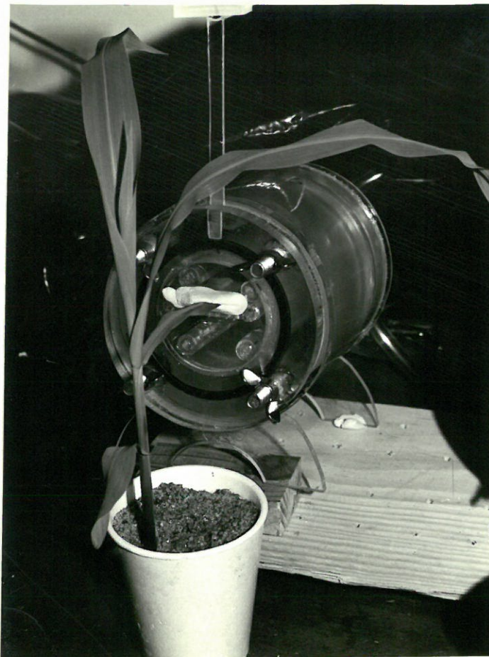
FIG. 1A Cuvette with leaf inserted showing Pres-stik sealing slit
