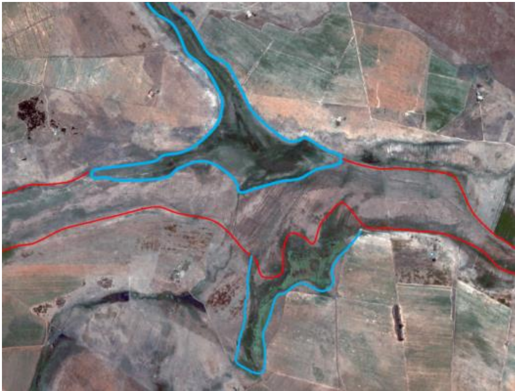
Figure 5.22: Different reflectance properties of wetlands may affect the outcome of the mapping process. Clearly discernible wetlands are indicated by the blue outlines, while those demarcated in red are less obvious wetlands. Different users may include the wetlands demarcated by the red outline while others users may exclude them (Note: the above image is for demonstration purposes only and is not considered to be a complete and accurate delineation of wetlands).
