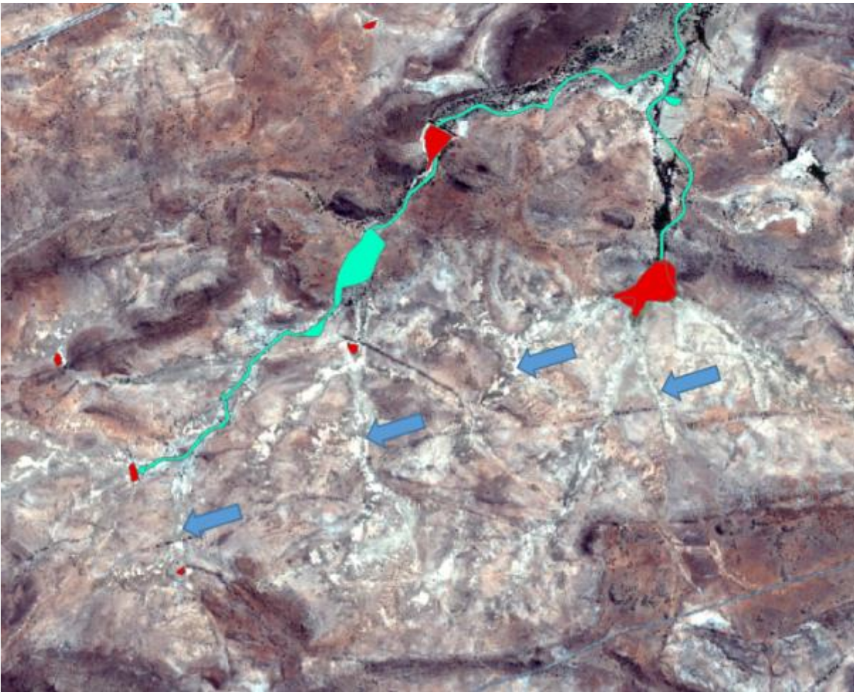
Figure 5.17: Valley floor areas in an arid area of high relief of which some portions of the valley floors were indicated to be possible wetland (cyan features) while others were not (blue arrow). The absence of vegetation from the valley floor areas requires the user to rely on expert knowledge on which areas, if any, are to be mapped as wetlands.
