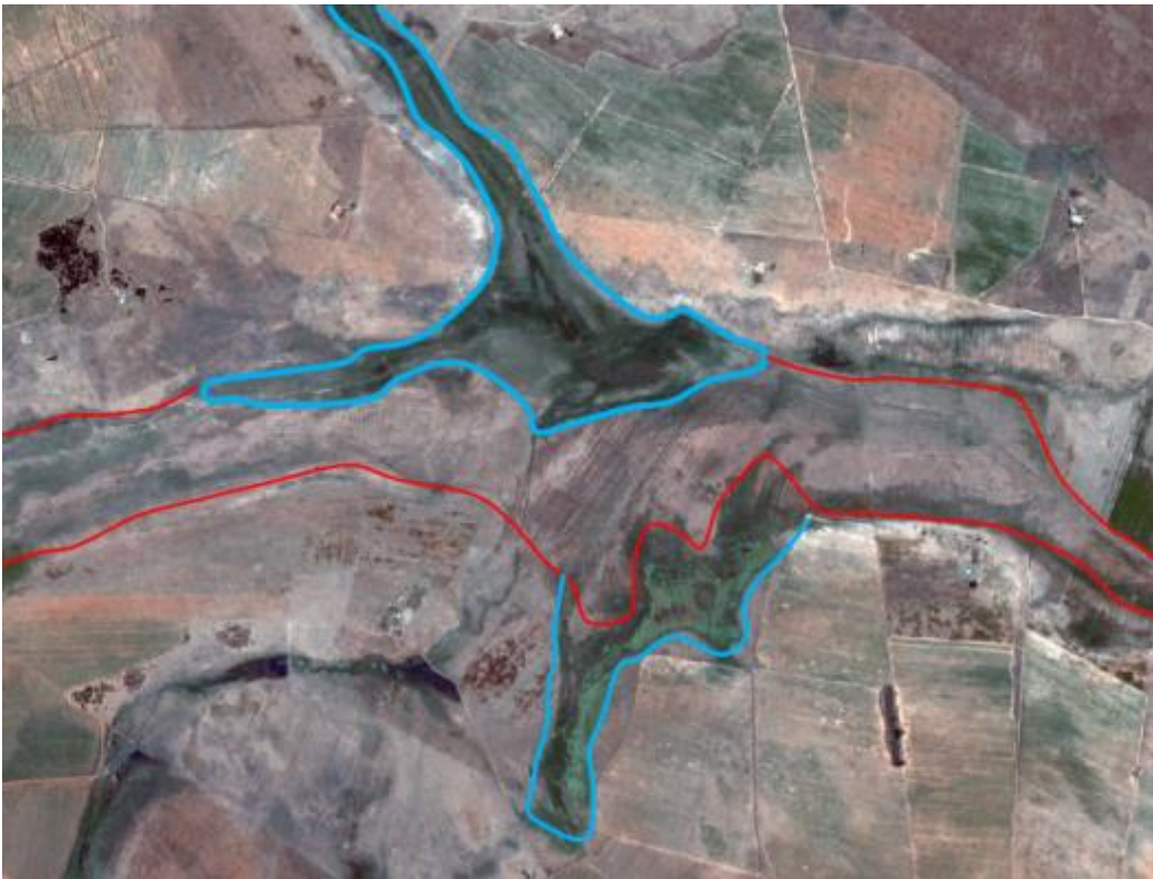
Figure 5.22: Different reflectance properties of wetlands may affect the outcome of the mapping process. Clearly discernible wetlands are indicated by the blue outlines, while those demarcated in red are less obvious wetlands. Different users may include the wetlands demarcated by the red outline while others users may exclude them (Note: the above image is for demonstration purposes only and is not considered to be a complete and accurate delineation of wetlands).
