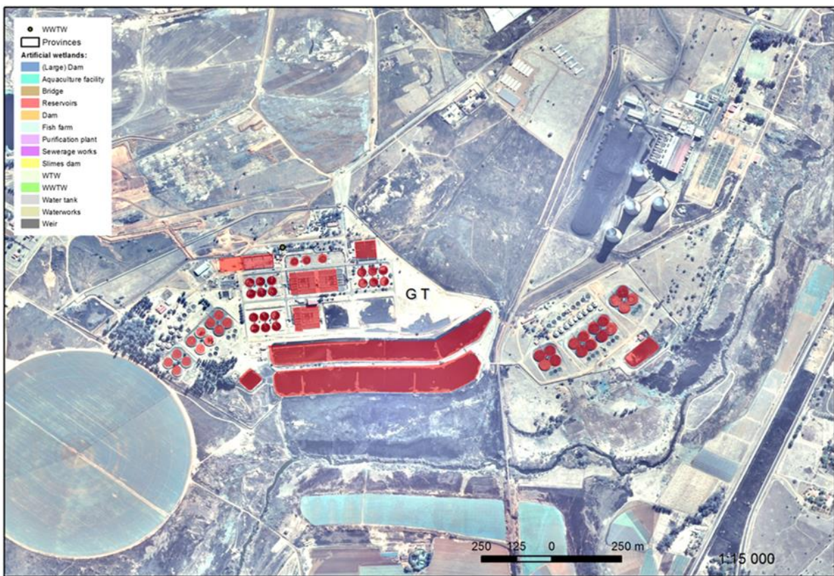
Figure 4.11: The extent of Waste Water Treatment Works (WWTW) as mapped by DRDLR:NGI.
