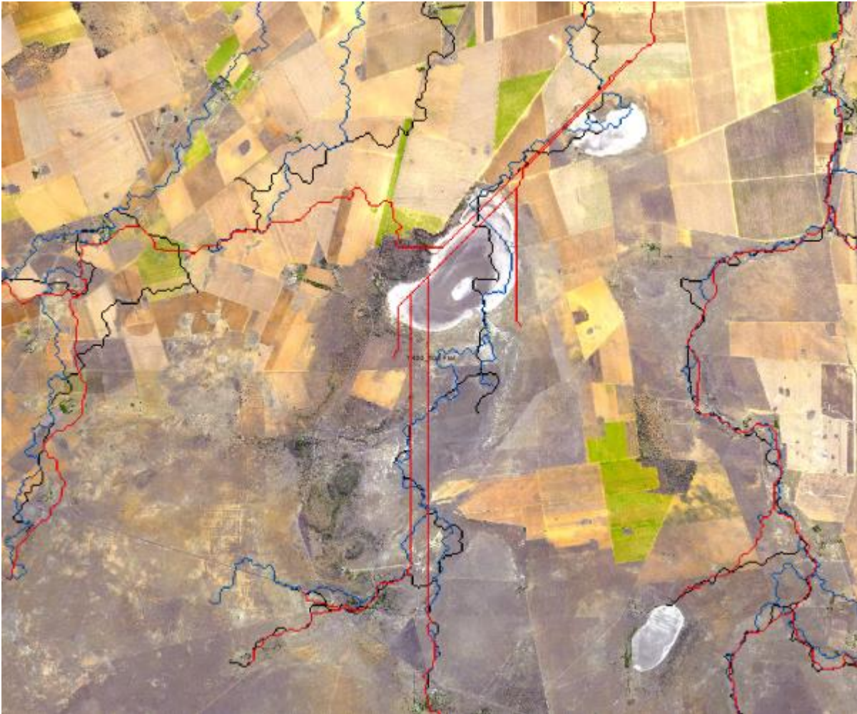
Figure 5.8: Comparison of flow accumulation outputs as derived from DEMs that were subjected to different methods of pre-processing. Red lines are flow accumulation derived from first applying the ArcGIS fill and then the flow direction and flow accumulation tools. Blue lines indicate flow accumulation derived from the Whitebox breach fast only tool with ArcGIS-derived flow direction and flow accumulation. Black lines indicate flow accumulation derived from the ‘breach’ and subsequently ‘breach fast’ tools in Whitebox GIS.
