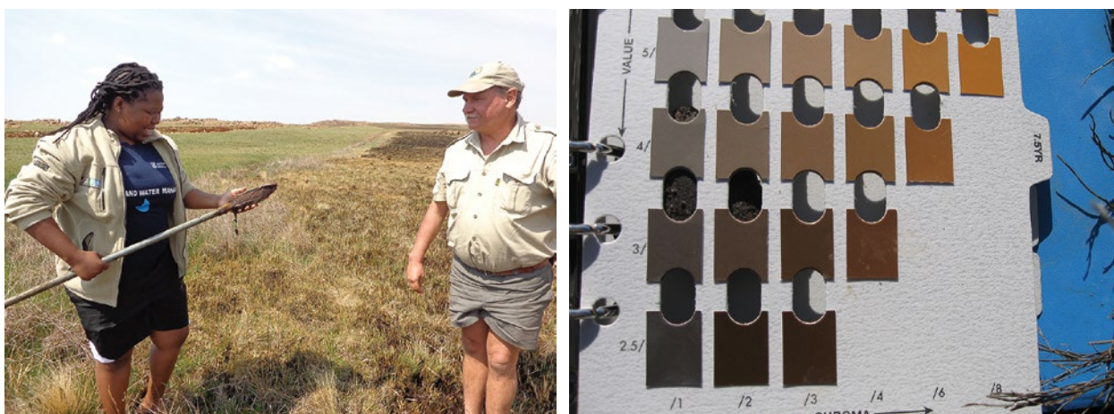
Figure 14: Soil information in the field can be collected with a soil auger (left) and matched against colours in a Munsell soil colour chart (right).
