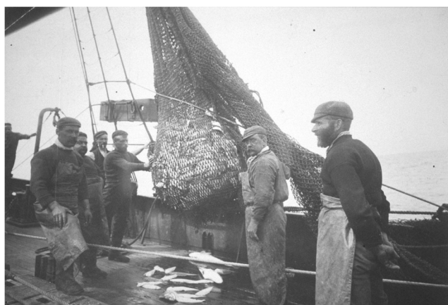
Fig. 4 Deck scene from the Pieter Faure, showing the full codend of the trawl. Mesh sizes and twine thickness were estimated from this photograph. DAFF Communications Archive Photo Library
