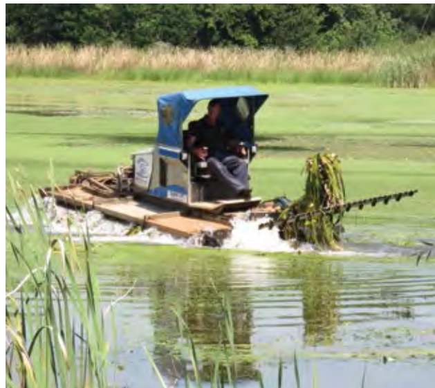
Figure 6. Use of an amphibious dredging machine to enhance the management of selected aquatic alien plant species in KZN.
